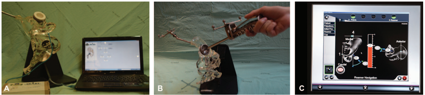
Figure 2. Experimental model setup. (A) Force-PRO device setup with software (A), computer-assisted navigation system (Orthopilot THA version 2.0, B. Braun-Aesculap, Tuttlingen, Germany) setup (B), and referencing information obtained from the alignment guide (C).
