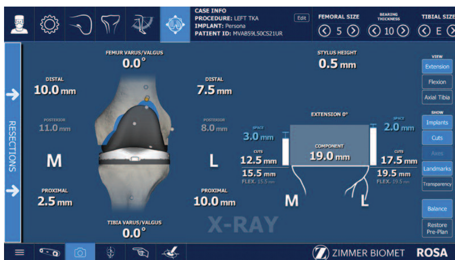
Figure 2a and b. Planning and modification of the angle and depth of bony resections using the ROSA Total Knee System.
